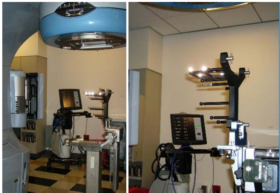
Fig. 2 A phantom of integrated target and fiducials was mounted either on the treatment couch ( right panel ), or on a BRW floor stand which can position the phantom near the isocenter with sub-millimeter accuracy ( left panel )
