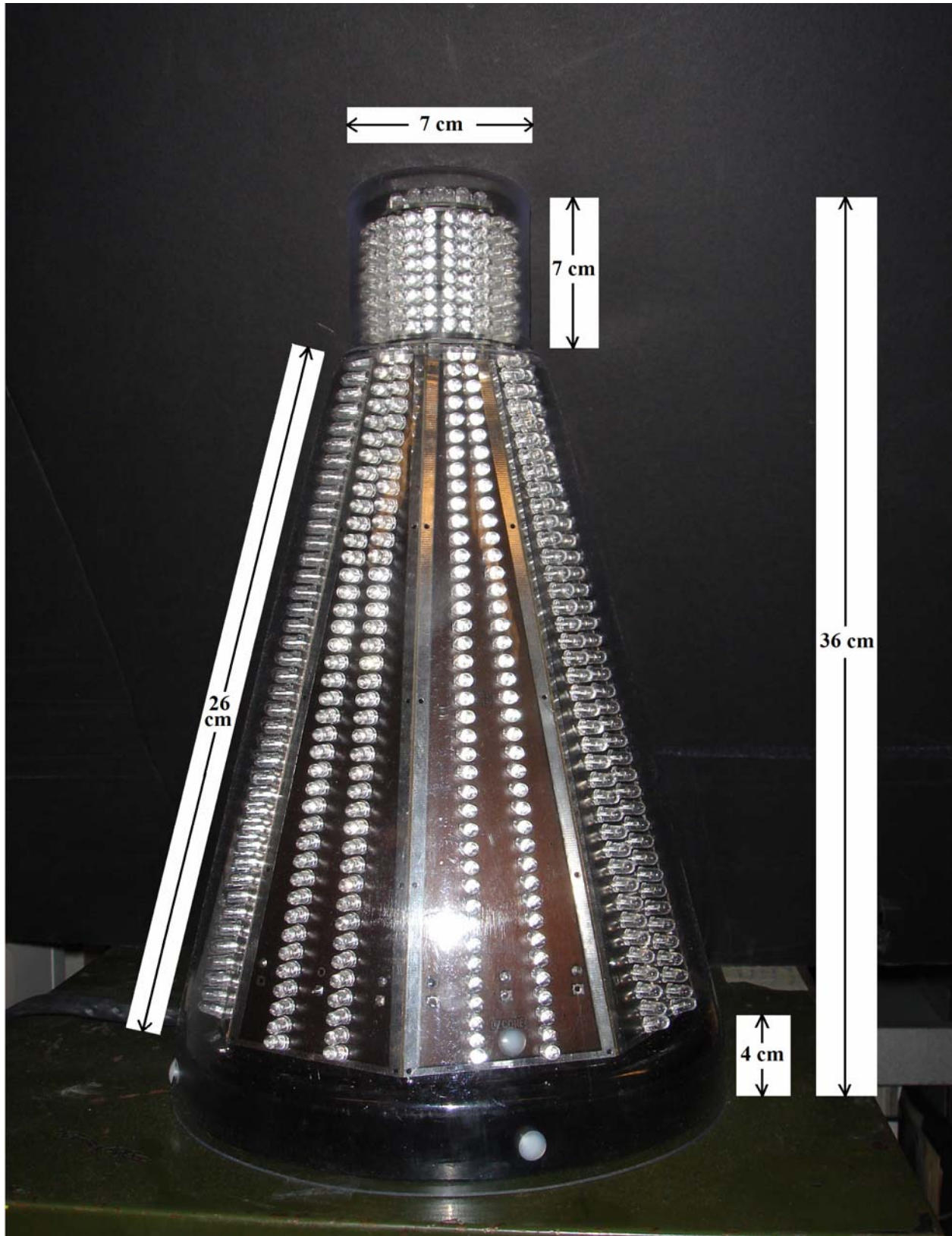
Figure 3: The truncated cone (lower portion) rests on a squat base cylinder that rises 4 centimeters. The “stripes”, two rows of LEDs on a trapezoidal circuit board, are 26 centimeters long. The overall height is 36 centimeters and the top cylinder has a ‘square’ profile—7 centimeters in height by 7 centimeters in diameter.
