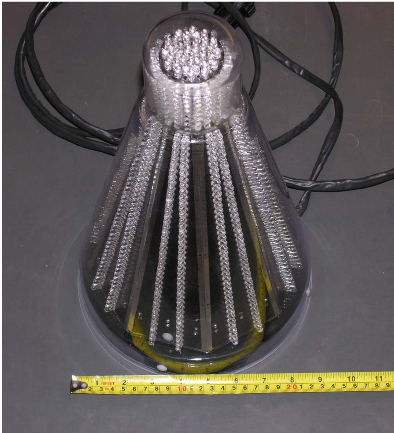
Figure 4: The base is 22 centimeters in diameter. There are 8 LEDs in a vertical column on the upper cylinder. There are 24 such columns ringing the cylinder. On the very top there are 36 LEDs forming a disk. Each line of LEDs on the truncated cone consists of 40 LEDs. Two such lines form a “stripe” on a trapezoidal board. There are 8 such stripes (or boards). The cord supplying power/control is seen in the background.
