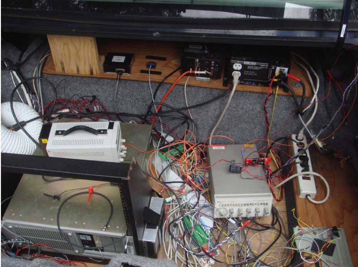
Figure 25: Radar support equipment occupies the trunk of the test vehicle.
