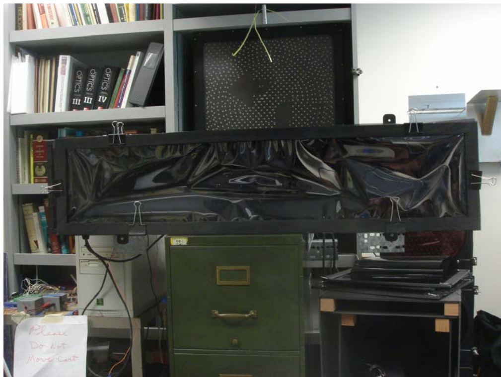
Figure 20: The configuration of attenuator and light bar as it was used for testing, except for the fact that the lower clips did not have their handles over the viewing surface; instead they pointed away from the surface like the upper and side clips.
