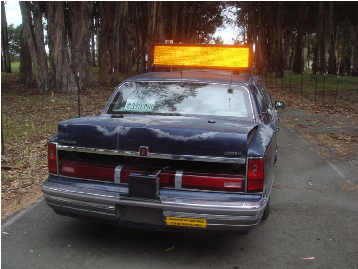
Figure 24: Test vehicle with shadow truck warning signal mounted and operational at the Richmond Field Station. The black rectangle (on the rear bumper just above the license plate well) with wires running into the trunk is the transponder for the radar unit.
