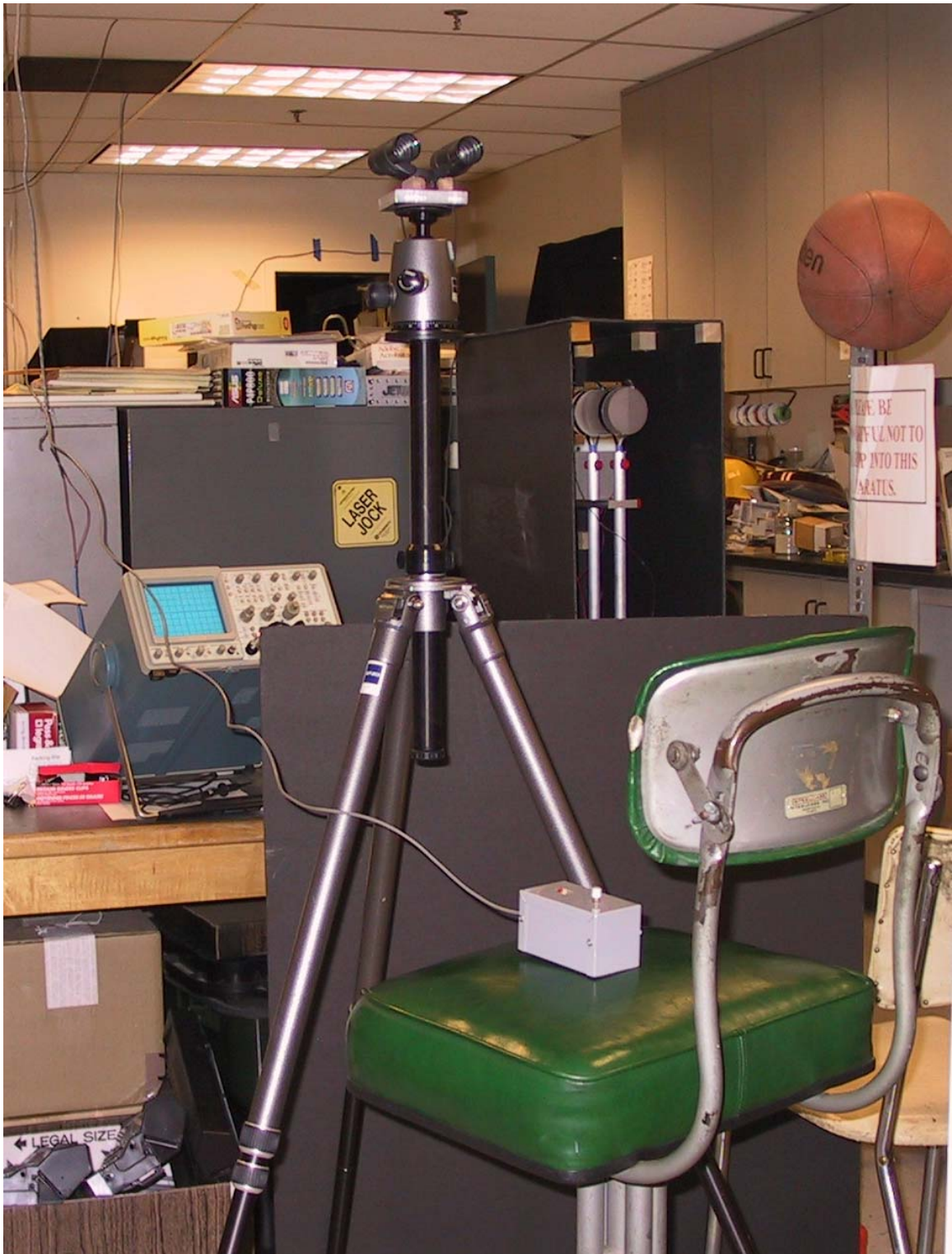
Figure 21: The subject's high chair and reaction time response button at the opposite end of the room about 25 feet from the light bar. (The inverted binoculars mounted on a tripod were not used nor present during the test.)
