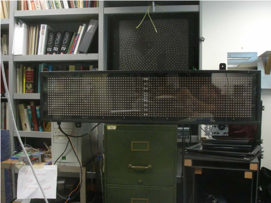
Figure 12: The prototype shadow truck warning light as mounted for testing. The light bar is securely bolted to angle iron framing that is mounted on the file cabinet (the angle iron is just visible on the upper right of the cabinet). The left-hand arrow signal behind the light bar is not relevant to this project.
