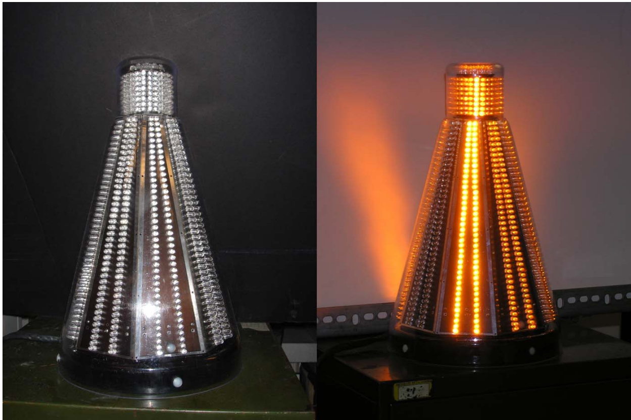
Figure 2: The final EWL prototype is shown unlit on the left and running in “inverted” mode (see text) on the right. Note the horizontal projection of the LEDs on the leftmost stripe of the unlit EWL and the amber/orange color of the LEDs in the lit view. The cone is held solidly to the metal file cabinet by its magnetic base.
