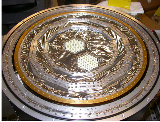
(a) The T-0 test setup consisting of wafer modules 8.2.0 and KT8 (closer to center) installed in the POLARBEAR receiver.
