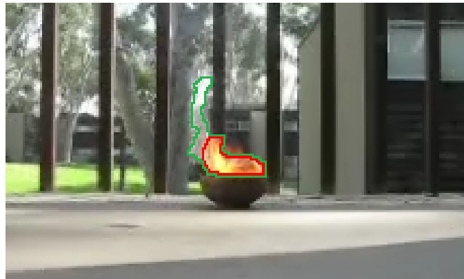
Figure 4.1: The green outline shows a hybrid fire-and-non-fire segmented output from the feature detection stage. The red outline indicates a “clean” segmented output from the feature detection stage.
