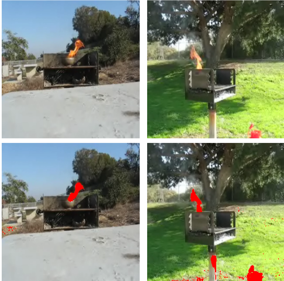
Figure 4.4: An example of fire color classification. The top row are the original images. The bright red color in the bottom row indicates where pixels have been classified as being fire colored.
