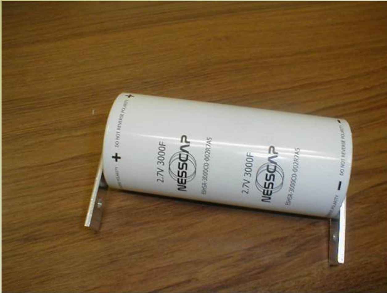
Nesscap 2.7V, 3000F Supercapacitor
