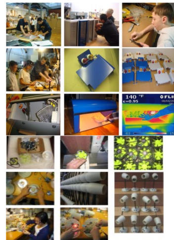
Figure 3.1.3-2: PCS fan + footwarmer, occupant's desktop interface, and manufacturing of 105 units
