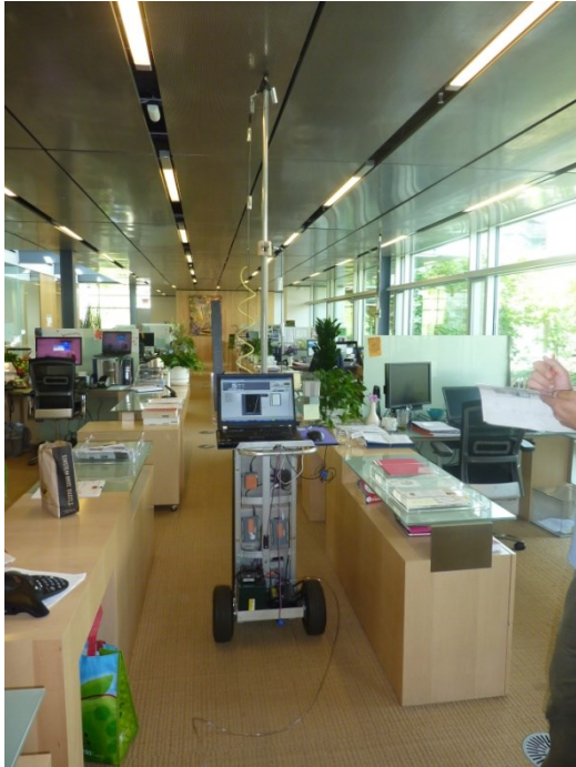
Figure 2.2.1-3: Stratification measurements and results display at Kresge Foundation
