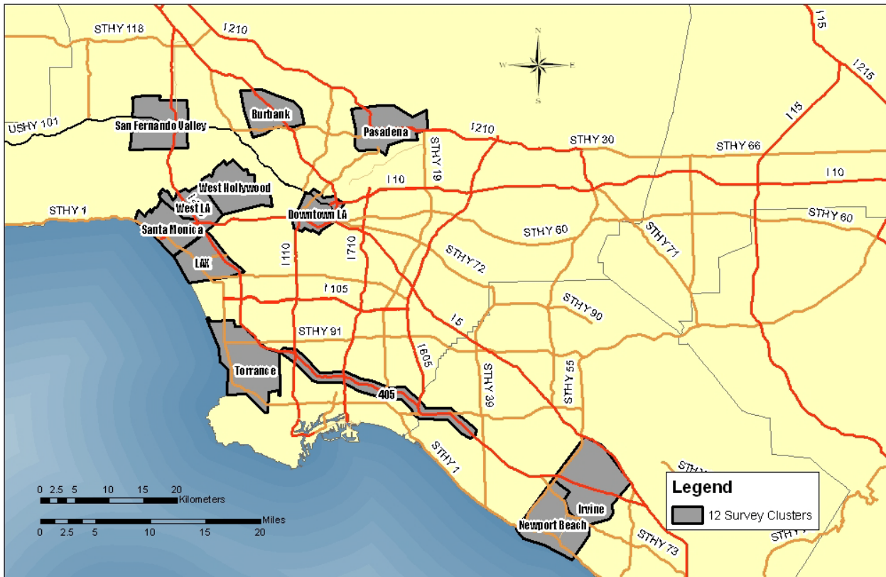
Figure ES-1 The shaded regions above are the “clusters” which are potential sites for early hydrogen vehicle and station placement. We used GIS analysis to evaluate scenarios where vehicles are introduced in 4 to 12 of these clusters between 2009-2017 to meet the requirements of the ZEV regulation.
