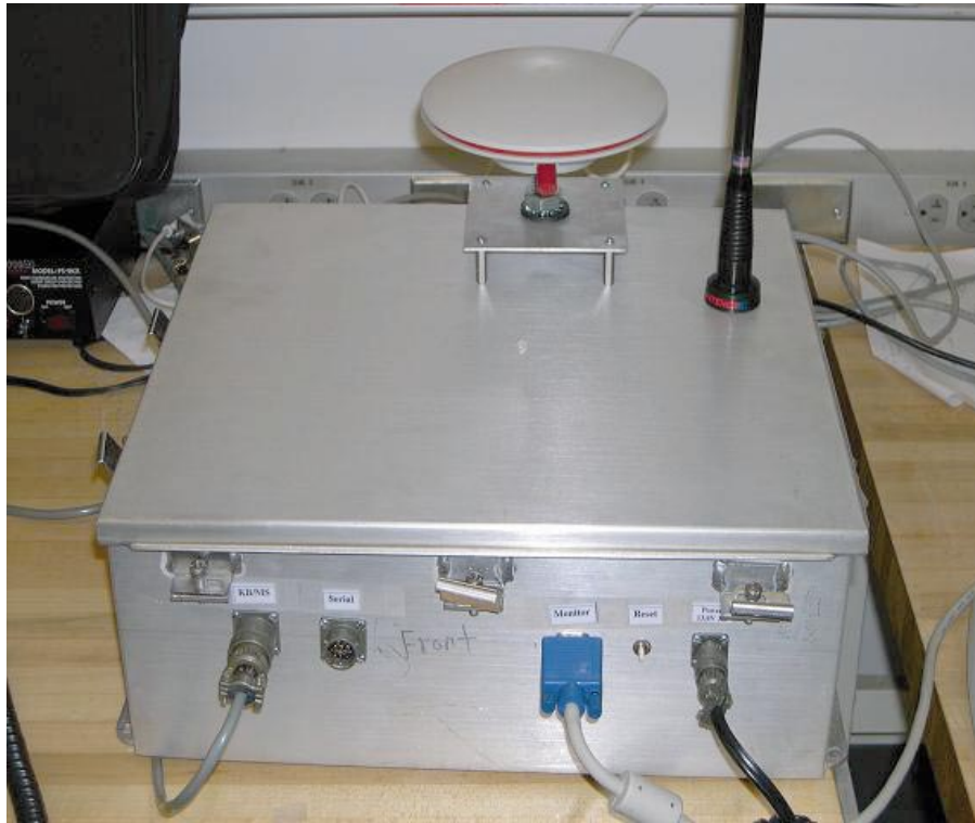
Figure 7: Photo of the outside of the GPS/INS prototype hardware box.
