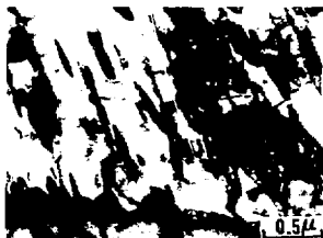
Fig. 5 Typical microstructure of the thermally stable \gamma_R at 77°K in 9Ni steel. \gamma_R particles are K-S related to the matrix of tempered \alpha' .
