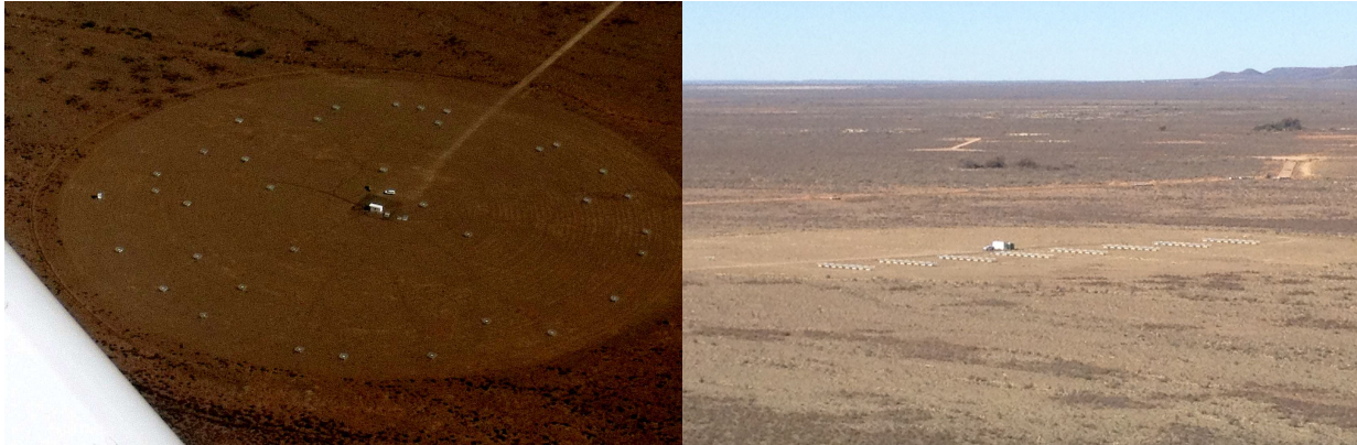
Figure 1.1: Left: Aerial photograph of a 32-element PAPER array deployed in a minimum redundancy configuration in May 2010. Right: Photograph of a 64-element PAPER array deployed in a maximum redundancy configuration in September 2012.
