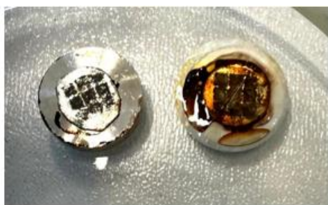
Figure 3-11: Opened anode half cells cycled in low salt concentration IL electrolyte (right) and high salt concentration IL electrolyte (left)
