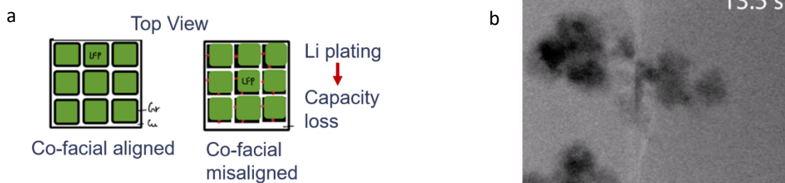
Figure 4-1: (a) Misalignment of the co-facial electrodes causing formation and growth of Li dendrites over time; (b) shorting of battery due to puncture of separator by the Li dendrites [37]
