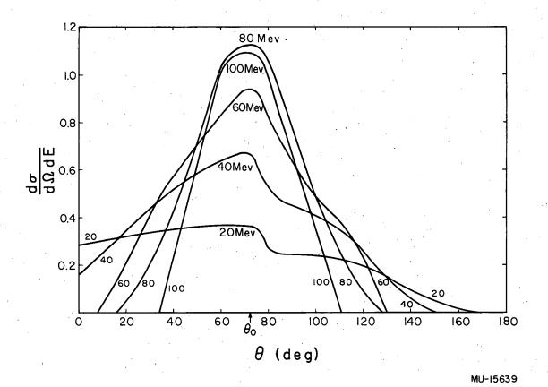
Fig. 2. The angular and energy distributions of nucleons emitted though the excitation of shock waves in nuclei by a very-high-energy incident particle. For the values of the parameters given in the text, the maximum energy for the emitted particles is about 115 Mev. The units of the ordinate are relative.
