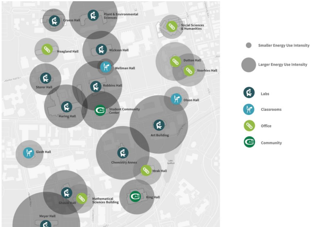
Figure 2. This map-based energy visualization, referred to as Icon Map, uses a colored icon to represent building type and grey circle of varying size to represent EUI.
