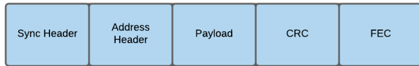
Figure 2.6. Representative structure of an underwater acoustic communication packet. Packets typically include a synchronization header, address header, payload, cyclic redundancy check (CRC), and forward error correction (FEC). Adapted from [17].
