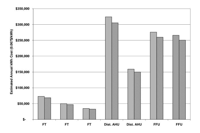
Figure 2. Projection of annual fan kWh cost (fans for air circulation) between year 2002 to 2020 for an 1,000,000 m<sup>3</sup>/h (or 583,000 cfm) Class 5 cleanroom
