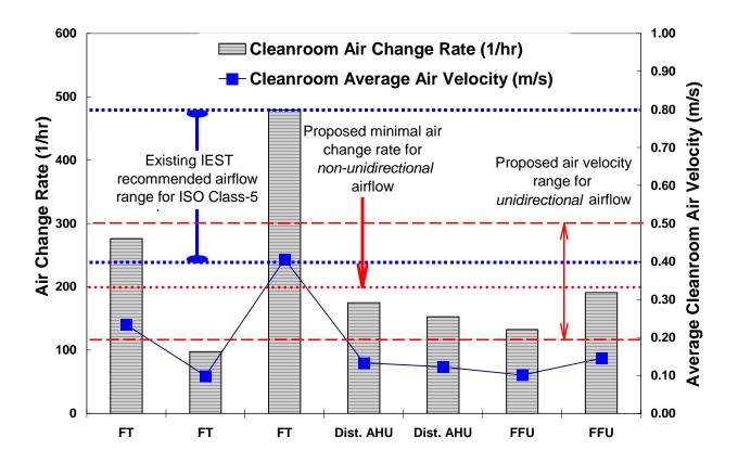
Figure 1. In-situ Class 5 average cleanroom air velocities and air change rates
