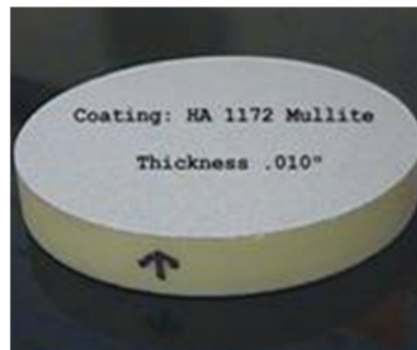
Figure 7.12: 50 mm alumina disk thermal spray coated with 250 \mu\text{m} thick mullite
