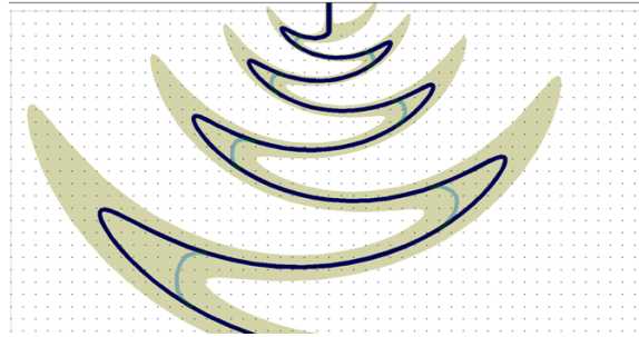
Figure 7.4: Suggestion for rerouting of transmission line on sinuous antenna. Current design follows sinuous antenna's curve (dark blue). By cutting corners as shown in light green, over all length of transmission line becomes shorter, and radius of curvature increases that would suppress reflection at corners.
