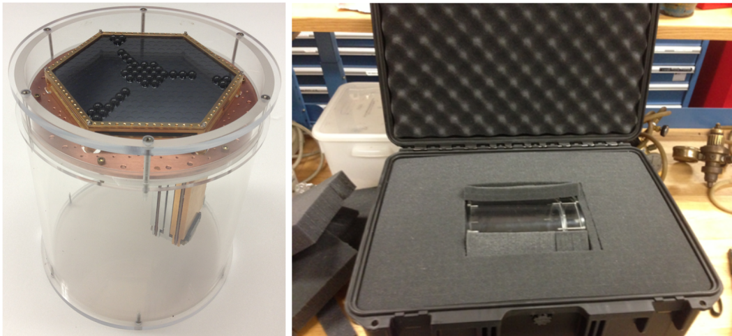
Figure 5.48: Photograph of plexiglass shipping container (left). Shipping container inside foamed case (right).
