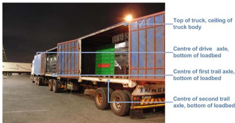
Figure 6.2: Typical location of accelerometers on typical South African truck.
