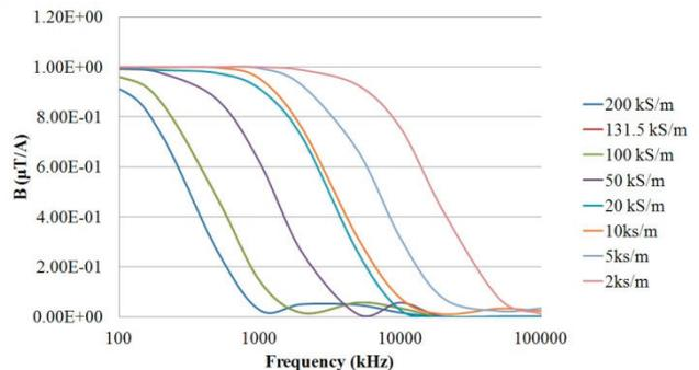
Figure 6: Pulse attenuation of the chamber vs frequency.
