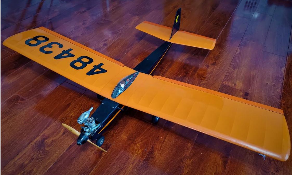
Figure 2.1: Carl Goldberg Falcon 56 Mk II R/C UAV reference vehicle.
