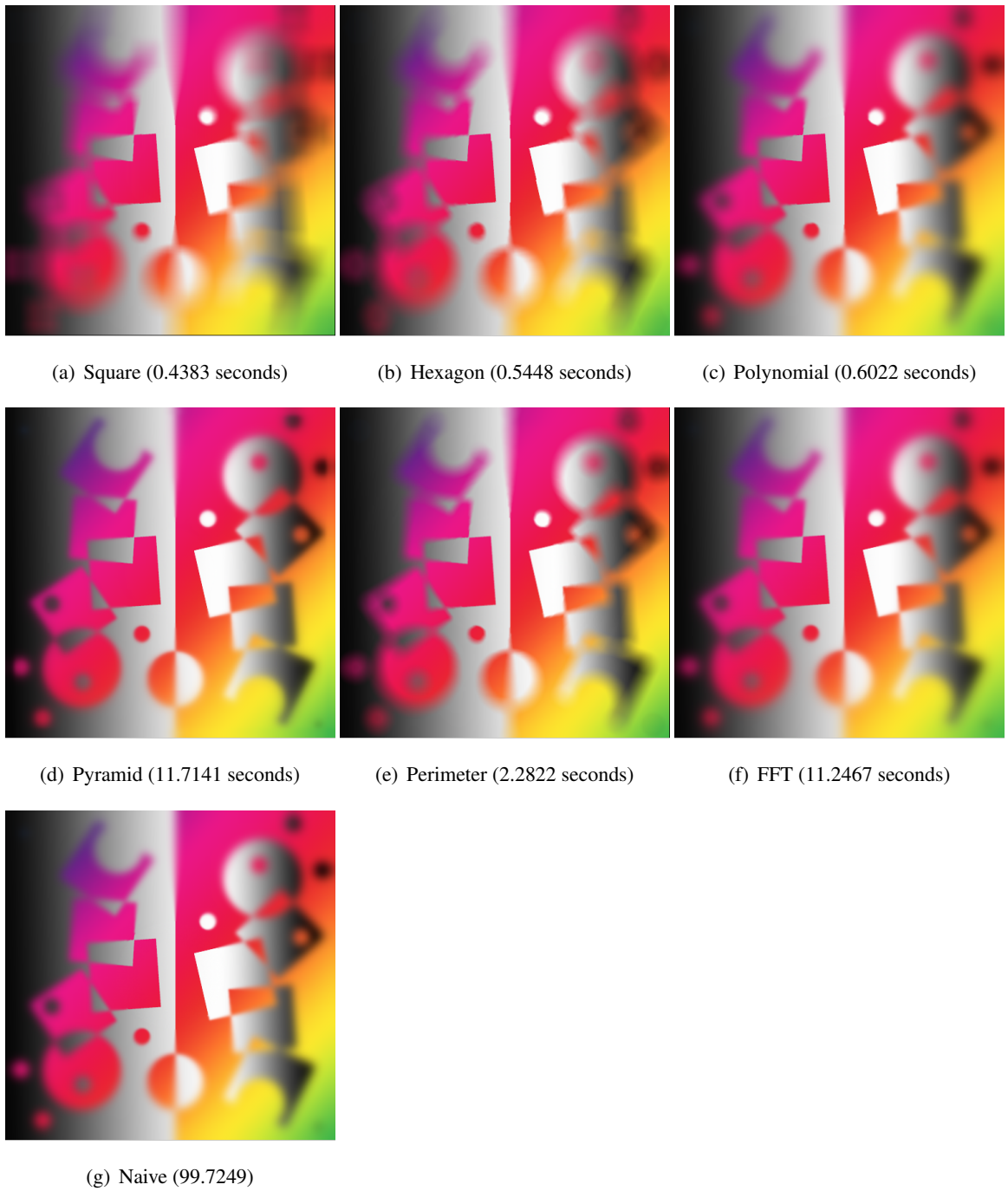
Figure 8.2: Various blur methods used on a low dynamic range image. Observe that each method produce similar result to the others.
