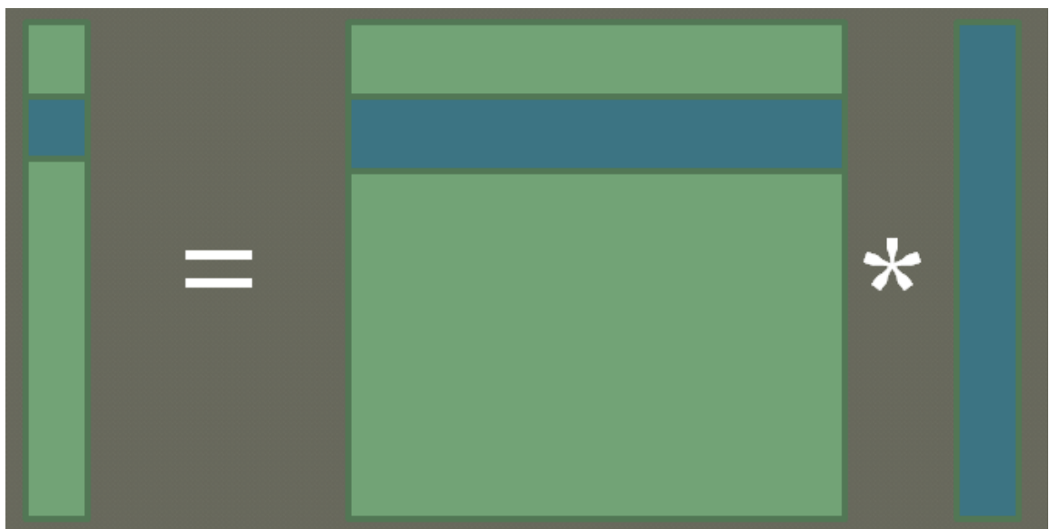
Figure 3.2: Matrix vector multiply can be implemented row-by-row. This corresponds to a gathering filter.
