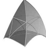
Figure 7: Ray casting of curved-quadratic tetrahedron T(u, v, w) having non-uniform density—where corner coefficients are zero and edge coefficients are one. Left image shows a rendering of the curved “faces” of T(u, v, w) . Right image shows ray casting of T(u, v, w) . Isosurfaces are for a small range of values near \{0.2, 0.575, 0.725\} . The “egg” corresponds to the isosurface at 0.725 and the corners correspond to 0.2.
