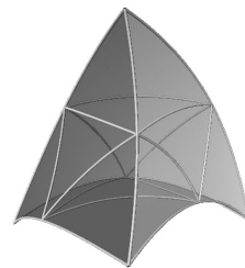
Figure 1: Example of a curved quadratic tetrahedron having ten control points; one for each corner and one at the midpoint of each edge. (Interior parameter lines, on the faces, are shown to indicate curvature.)
