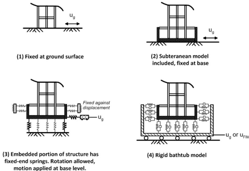
**Figure 2.** Schematic illustration of simplified models 1 to 4 considered in simulations.
