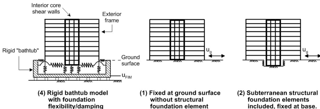
**Figure 5.** Schematic illustration of modeling approaches for the Walnut Creek building.
