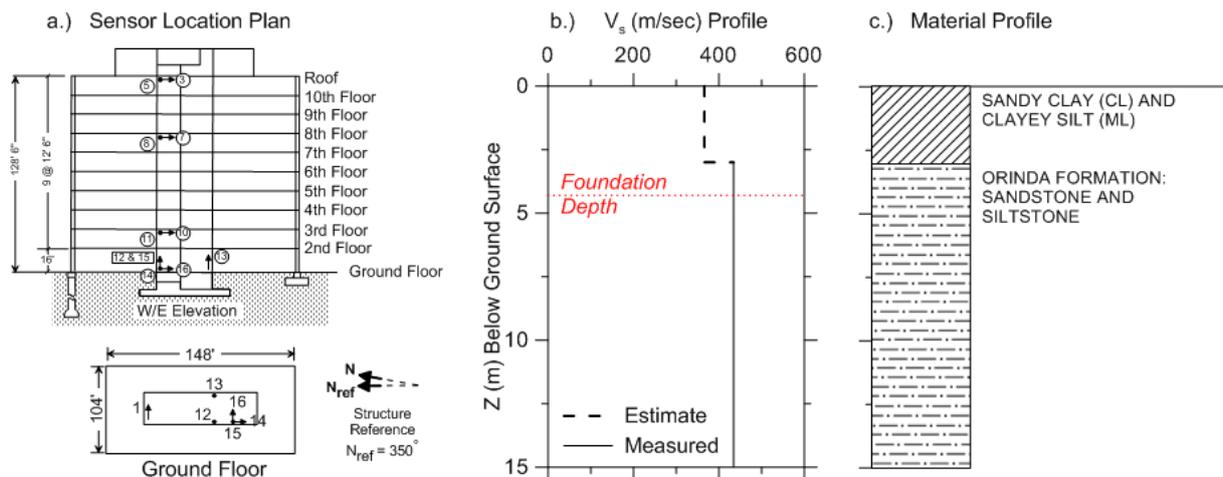
**Figure 4.** Illustration of Walnut Creek building and site characteristics; a) foundation and east-west oriented building sensor location map, b) soil shear-wave velocity profile, and c) soil material profile description.
