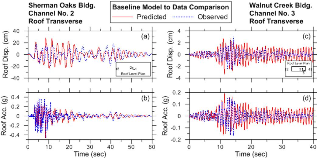
**Figure 6.** Comparison of baseline model and recorded roof response histories for a) Sherman Oaks building absolute displacement, b) Sherman Oaks building absolute accelerations, c) Walnut Creek building relative displacement and d) Walnut Creek building absolute acceleration.
