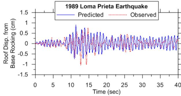
**Figure 7.** Comparison of roof displacement due to base rotation of baseline model and recorded data for the Walnut Creek building.
