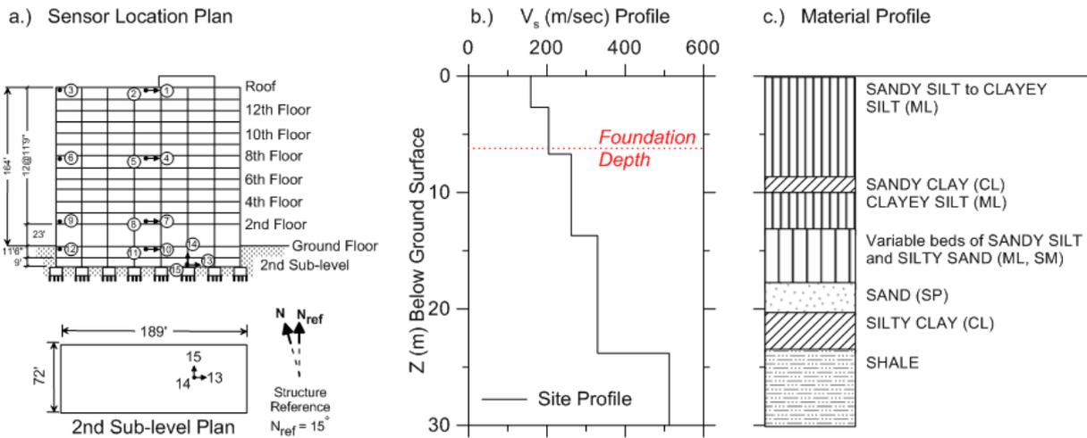
**Figure 3.** Illustration of Sherman Oaks building and site characteristics; a) foundation and east-west oriented building sensor location map, b) soil shear-wave velocity profile, and c) soil material profile description.
