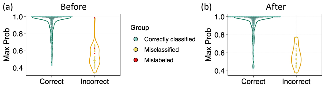
Figure 4.5: Maximum predicted probability for correctly and incorrectly predicted samples of all diblock copolymers using the physics-informed features for (a) the original samples; (b) revised samples after correcting three mislabeled detected by our method.
