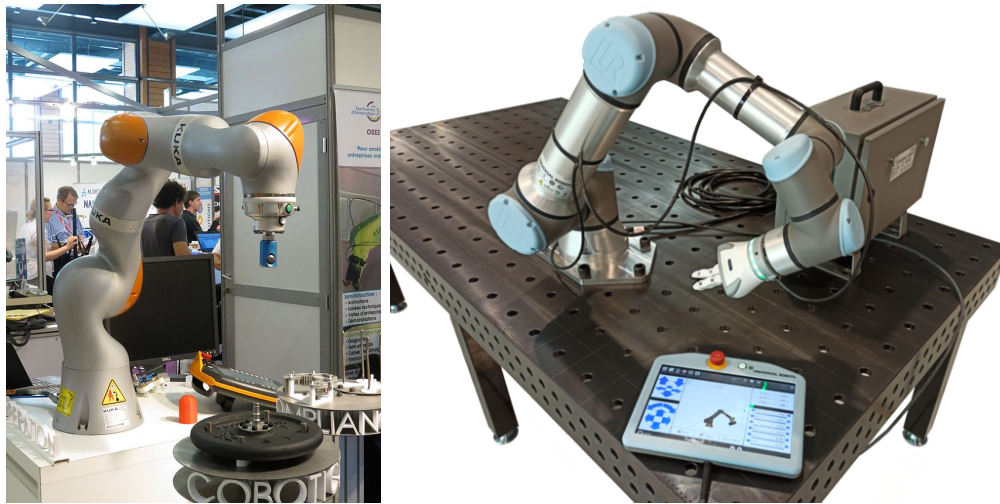
Figure 2.1: Two modern collaborative robots, or cobots , designed for human-robot interaction. On the left is KUKA 's LBR iiwa and on the right is the Universal Robots ' UR16e. Each manipulator is instrumented with integrated force-sensing to detect forces in operation.
