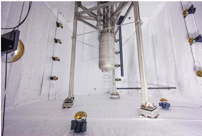
FIG. 4. Photograph of LUX installed in the Davis Cavern water shield at SURF.
