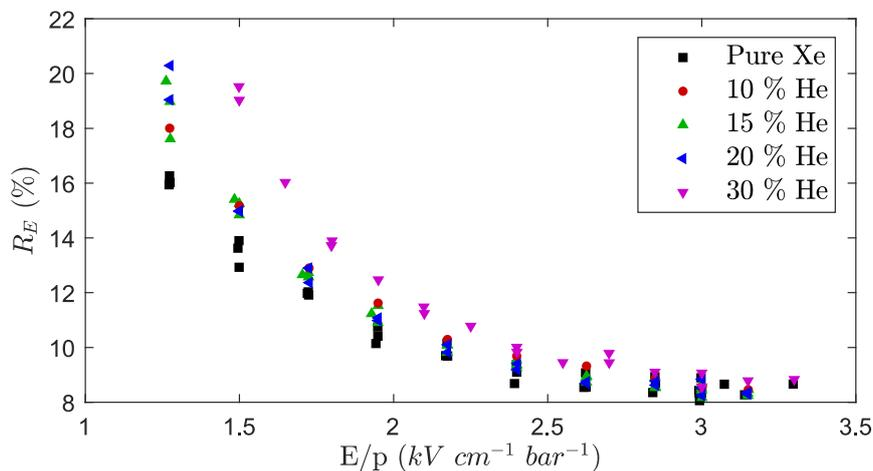
**Figure 10.** Energy resolution as a function of reduced electric field in the EL region, obtained for pure xenon and the different Xe-He mixtures studied in this work. A relative statistical error of 3% was calculated for several measures having the same working conditions.
