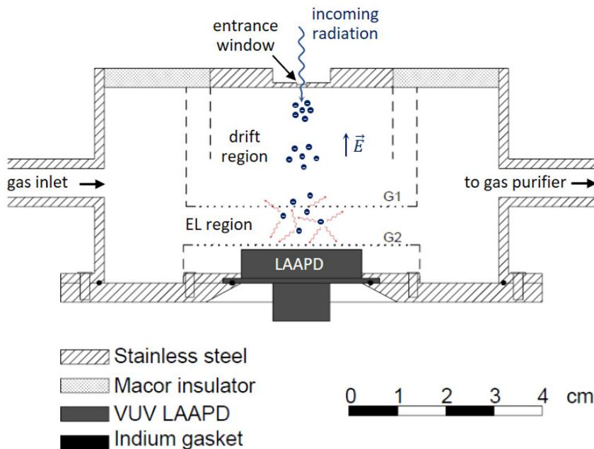
**Figure 2.** Schematic of the Gas Proportional Scintillation Counter used for this work. A VUV-sensitive LAAPD is used as photosensor and the gas is continuously purified, circulating by convection through SAES St707 getters.
