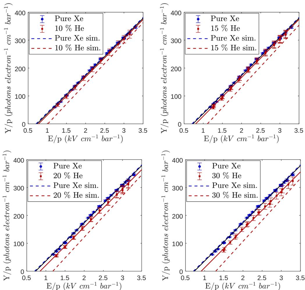
**Figure 8.** Reduced electroluminescence yield as a function of reduced electric field in the EL region for pure xenon and the different Xe-He mixtures studied in this work. Solid lines show linear fits to the experimental data, while dashed lines are the simulation data obtained with the simulation tool of ref. [33].
