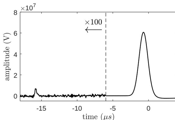
**Figure 6.** Typical average waveform produced by alpha particles (a few tens of Hz) in pure xenon at 1.1 bar, for a mean reduced electric field of 376 V/cm/bar in the drift region, and a reduced electric field of 2.7 kV/cm/bar in the EL region.
