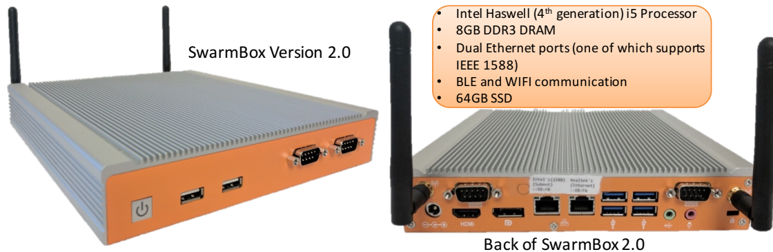
Figure 2.4: The TerraSwarm SwarmBox 2.0 edge computing server is hosted in IMB-186-4300U manufactured by ASRock Inc.
