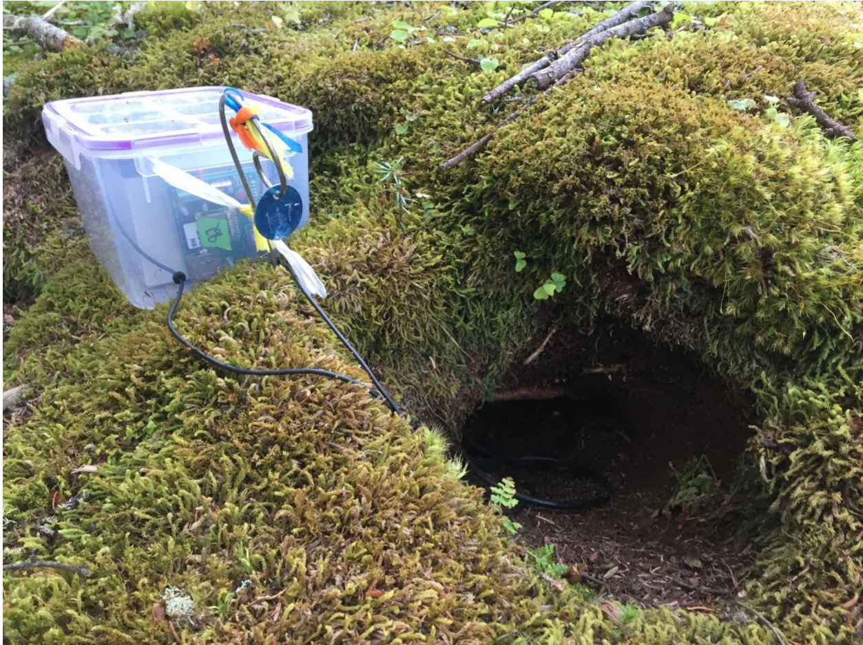
Figure A1.1 RFID reader and battery housed in waterproof plastic food storage box with two antennas placed in the burrow entrance. The first antenna is visible within the burrow opening.
