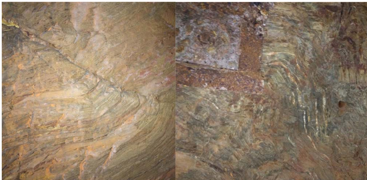
Figure 2.6. Folded and fractured schist of the Poorman Formation in first cross drift in 17 Ledge area, 4850 level. Photos are approximately 1 m across (left-hand image) and 0.5 m across (right-hand image).
