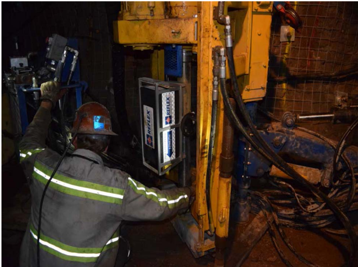
Figure 2.12. Orienting the drill pipe at the start of kISMET-004 using the REFLEX gyrocompass.
