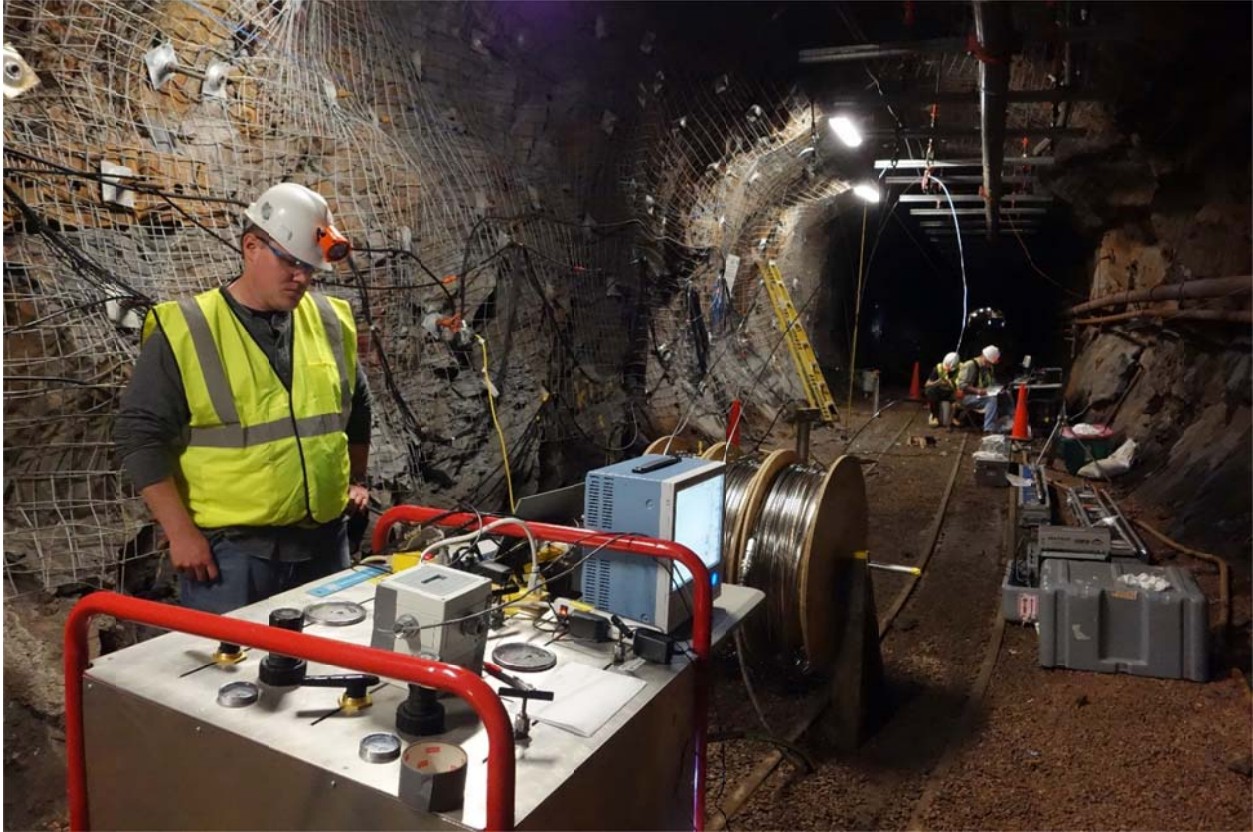
Figure 5.8. Pressure generators and digital data recorders used for hydraulic fracturing and fracture stimulation at SURF.
