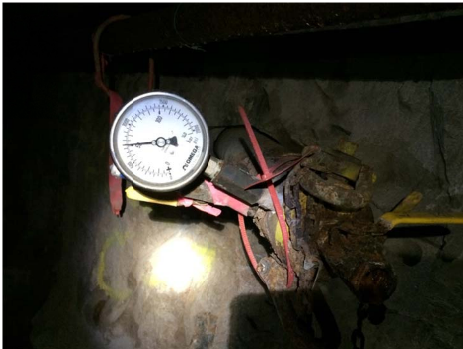
Figure 2.5. Instrumented drill hole with a static pressure of 700 psi (50 bars) at Drill Station 2.
