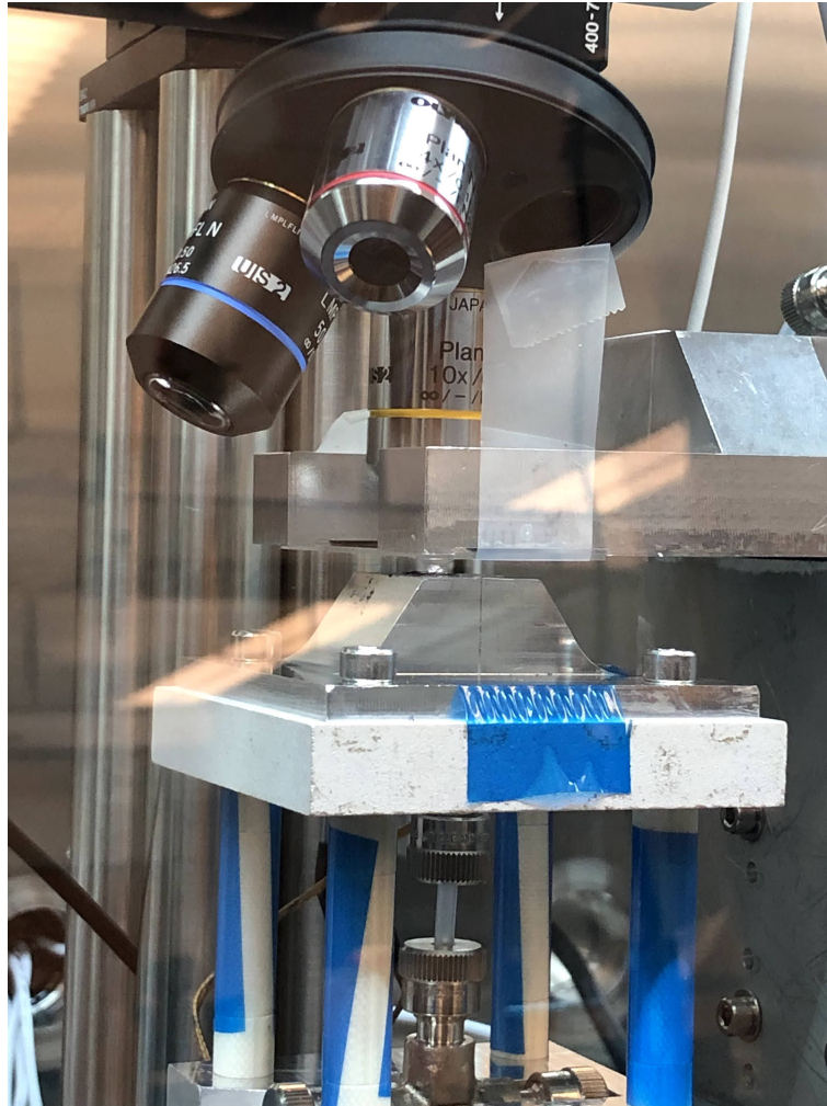
Figure 2.4: Custom-built Transfer Microscope inside Glovebox
