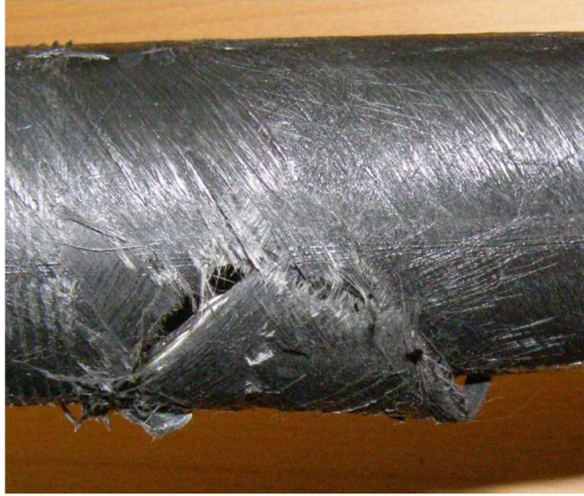
Figure 1.8. Burst under internal pressure [22]
