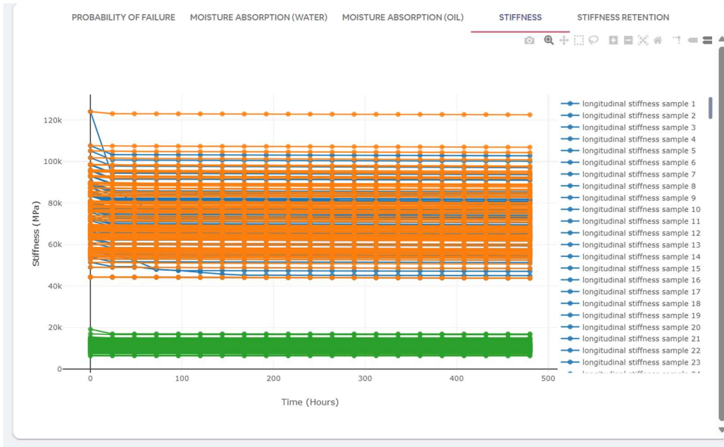
Figure 10.6. Stiffness value results for each sample in all three directions. When many samples are simulated, a large amount of data will be presented on this graph, which may make difficult to read. In this case the user can hide individual results by clicking on the name of the curve using the legend on the right.
