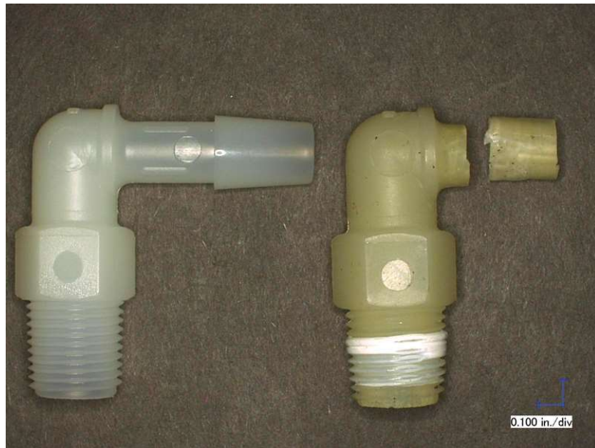
Figure 1.14. UV Degradation of a plastic part [38]
