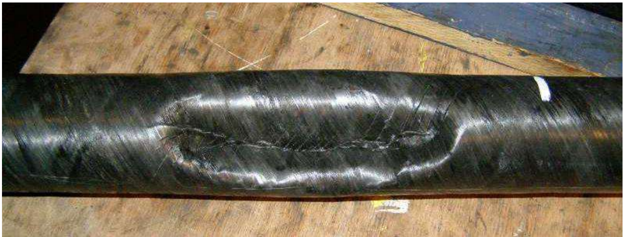
Figure 1.9. Collapse under external pressure [22]
