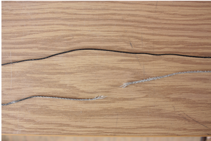
Figure A.3: This figure shows wear on the cable. The vectran cable's protective outer coating wears off during use which then allows for the individual fibers to break weakening the entire cable. Eventually this wear will degrade the max holding tension to the point of failure. The black cable is a new vectran cable and the cable below shows the black coating worn away and a breakage point. The bottom cable is from an actual failure on the system during a run. Since the system can absorb forces, when the cable breaks the stored energy gets distributed into the robot and no violent backlash is experienced.
