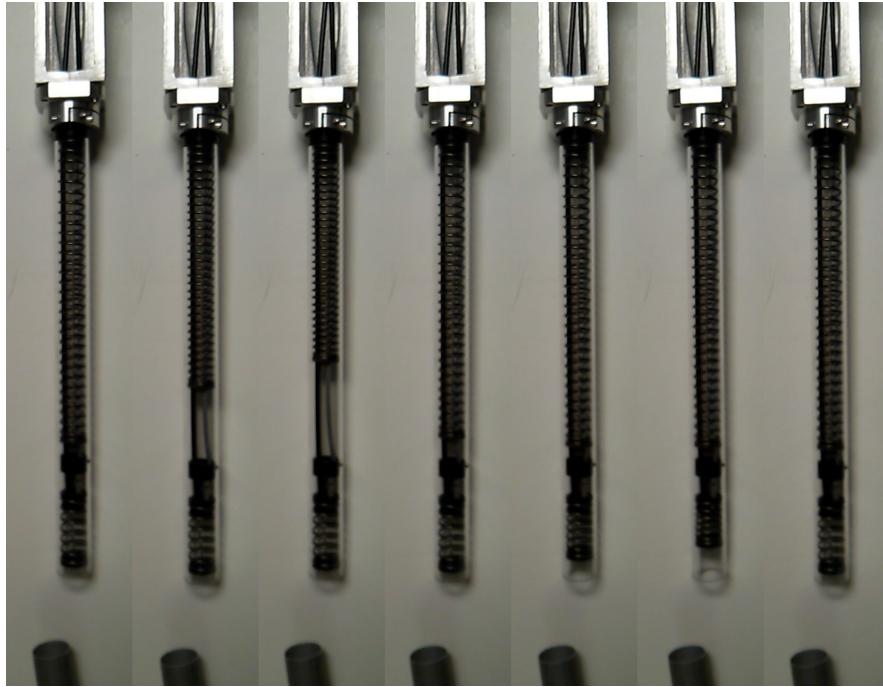
Figure 4.2: Time lapsed stills of spring compression in the MTR spring holder. Note that these stills are from a previous version of the MTR.
