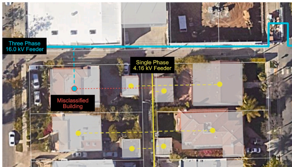
Fig. 2. Example illustration of the results of an automated building-to-circuit assignment procedure based upon minimum Euclidean distance, with an evident misclassification error shown.
