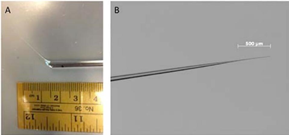
**Figure 2. Preparation of glass needle for surgery.** (A) Needle is drawn from the end of a solid glass rod. (B) High magnification view of needle tip indicating the length and sharpness necessary for surgery. [Click here to view larger image.](#)
