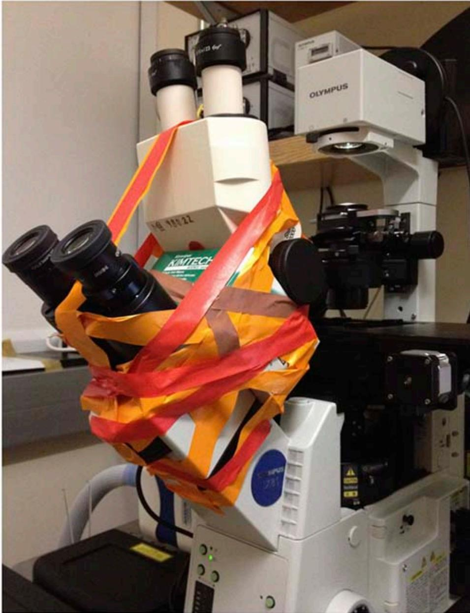
**Figure 4. Double-decker microscope configuration.** A dissecting microscope head is mounted on top of the eyepiece head of an inverted microscope. Lab tape allows the apparatus to be rapidly assembled and disassembled when the experiment is completed. [Click here to view larger image.](#)
