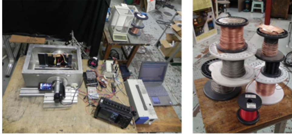
Figure 3.1: Photo of test stand (a) test platform, (b) sample wires.
