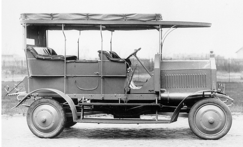
Figure 1.3: ‘Dernburg-Wagen,’ the worlds first all-wheel drive passenger car which also features RWS [2].
