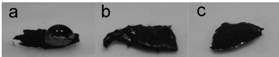
Fig. 1. Wetting of (a) CF; (b) Na-ACF and (c) K-ACF.
