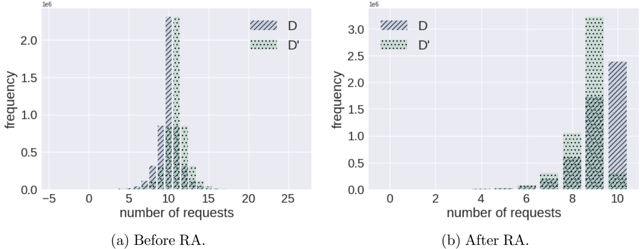
Figure 4.4: Distribution of output over 5 million runs. Before RA, we draw noise from a double geometric distribution with \epsilon=1 and k=10 . After RA, the distribution changes, and the privacy leakage increases (the empirical \epsilon rises to 2.07).
