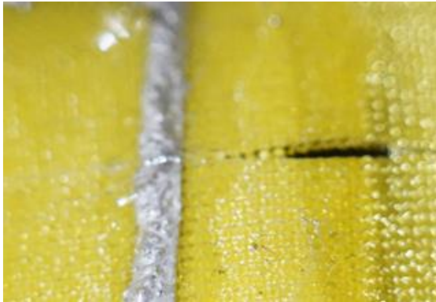
Figure 13. Man-made Crack on MLM Dynamic Circuit.
