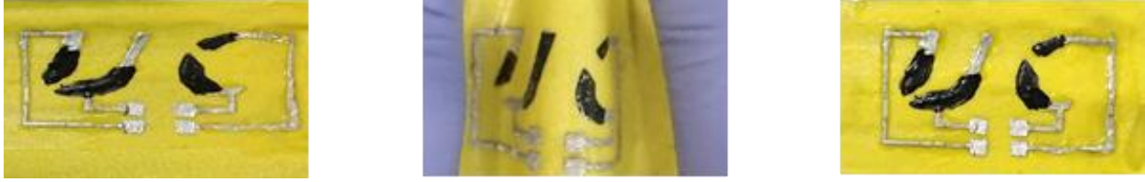
Figure 12. Stretching test (left), bending test(middle), and the Rest (right).
