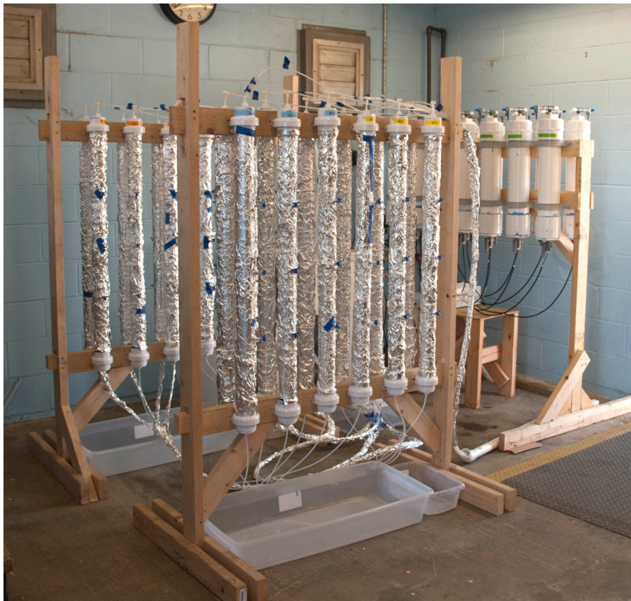
Figure 5.2 One-meter columns of mixed geomedia in various configurations testing geomedia performance and aging in authentic stormwater at a Sonoma, CA field test site.
