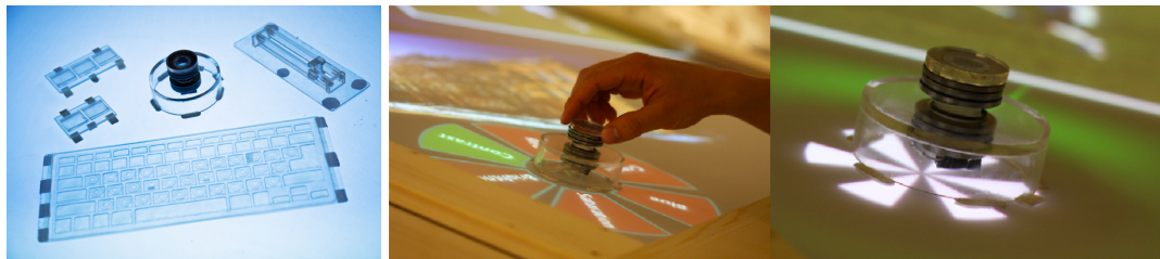
Figure 2.6: Slap widgets for an FTIR table. Images borrowed from Weiss et al. (2009).
