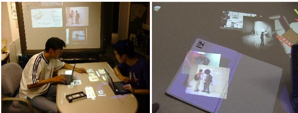
Figure 2.3: Jun Rekimoto's Augmented Surfaces supports fluid interaction between multiple devices and between digital and physical materials.
