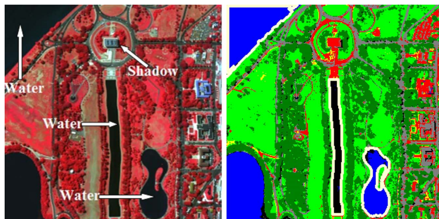
Fig. 2. Example of land cover with similar spectral properties being misclassified. (a) Original image. (b) Classified and segmented result. Note that the water part in the middle is misclassified as shadow.
