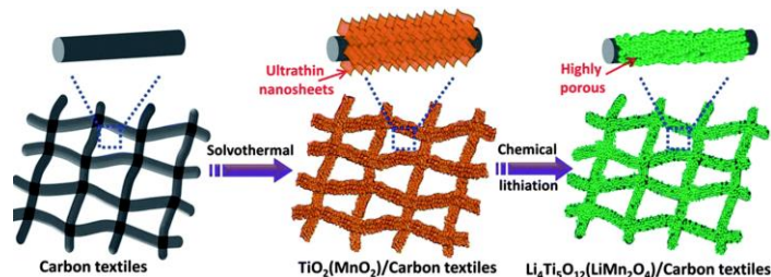
Figure 1.9 Schematic of the fabrication of lithium metal oxide/carbon textile composites. 41
