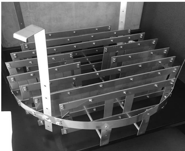
Figure 2.1. Custom stainless-steel coupon holder with some coupons inserted. The height of the apparatus can be adjusted to latch onto the outside of fermentor and position coupons in the cap of the fermentation.
