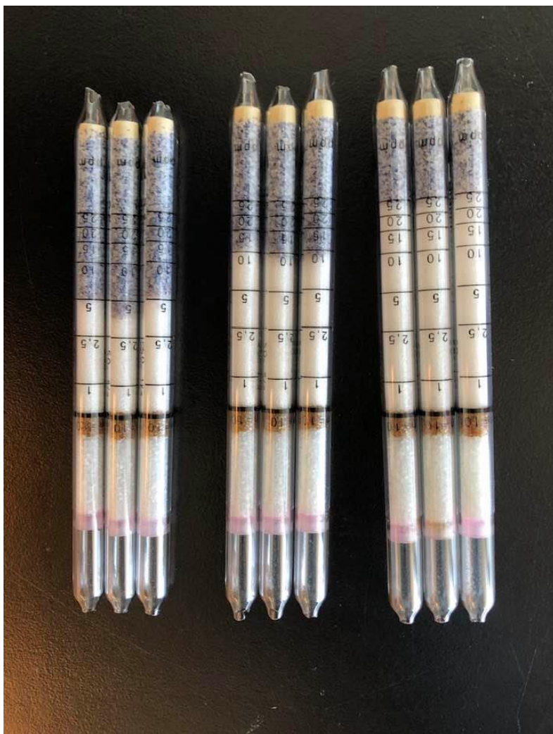
Figure 5.2. Dräger GDT calibration response. The extent of bleaching indicates sulfur dioxide concentration using the pre-indicated scale (in ppm). Concentrations converted according to Eq. 5.2 and Eq. 5.3 for 12.7°C cellar conditions.
