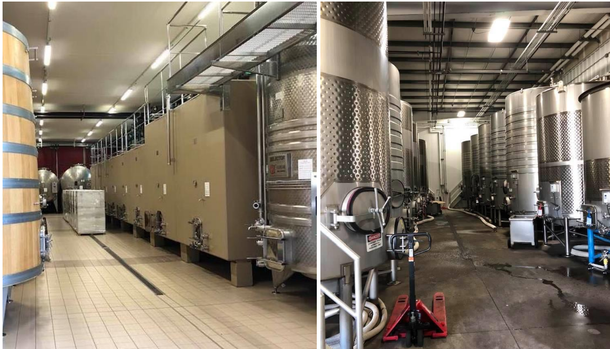
Figure 1.1. Variability of inert tank sizes and materials used in wineries. Left: SS, lined concrete, and lined wooden vats in an Italian production facility. Right: A variety of SS tanks sizes and configurations in an American winery. Photographs taken by author.
