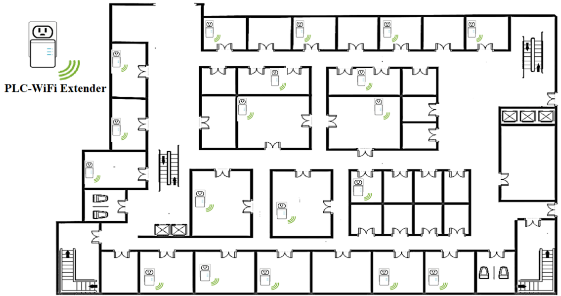
Figure 2.1: Powerline communications extend WiFi coverage through existing interior power lines in a home/enterprise.
