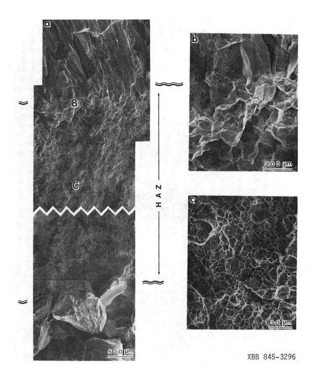
Fig. 5 - SEM fractographs showing (a) the fracture mode change occurring from weld metal to base metal, (b) and (c) are the magnification of the areas maked B and C, respectively in (a).
