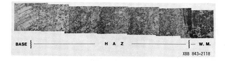
Fig. 4 - Optical picture of bead-on-plate weldment showing the distinguishable change in microstructure across the HAZ.
