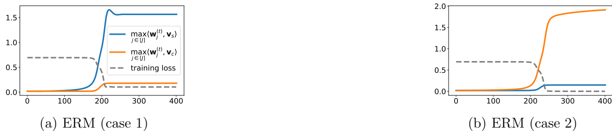
Figure 9.10: Training process of ERM trained with GD+M. We consider the same dataset generated in Figure 6.4 and observe almost the same training process as ERM with GD, except GD+M learns the features faster.
