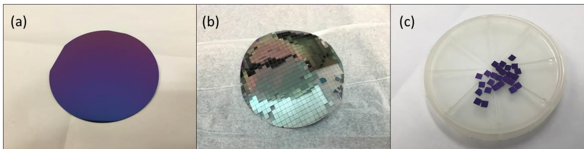
Figure 7.1. (a). 4 inch Si/SiO 2 wafer. (b). Laser-diced small chips with protective coating layer. (c). Clean square chips.
