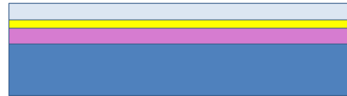
Figure 3.1. Si (blue) /SiO 2 (purple) wafer with Cr (yellow) layer and PMMA resist layer.
