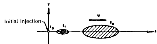
Fig. 1. Bidimensional flow, migration of the tracing spot after a brief injection.
